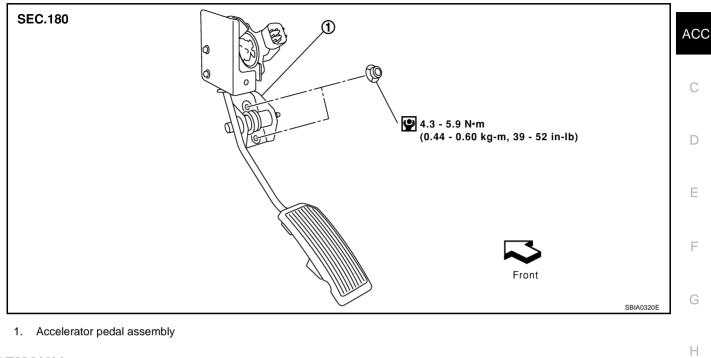
**REMOVAL** 1. Disconnect accelerator pedal position sensor harness connector
